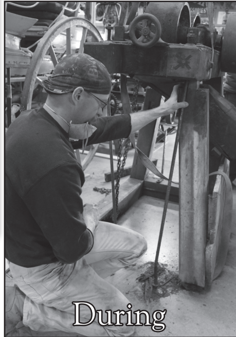
Jem Blueher repairing the mill's rotted legs in his Anvil Wagon Works shop
